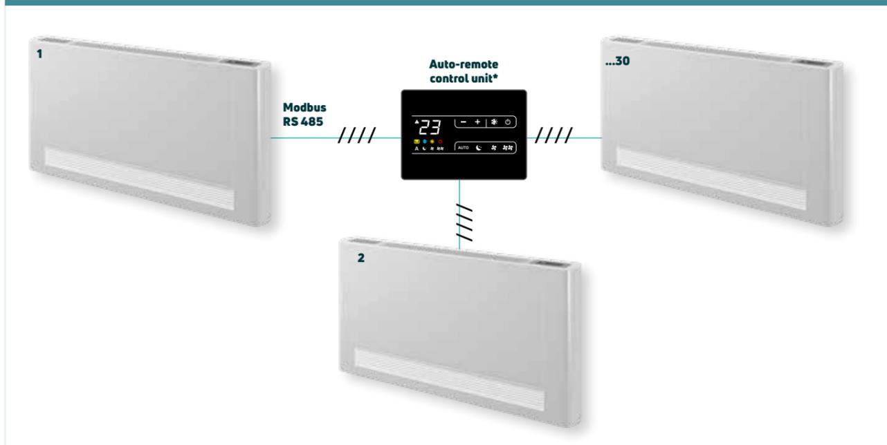
\* a single remote controller can control up to 30 Auto Remote iVector S2 devices
